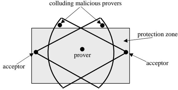
Fig. 3. Verifying prover's location using directional antennas. Defeating verification by colluding malicious provers.
