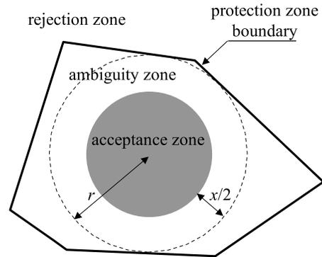
Fig. 1. Zone delineation for case of a polygonal protection zone.
