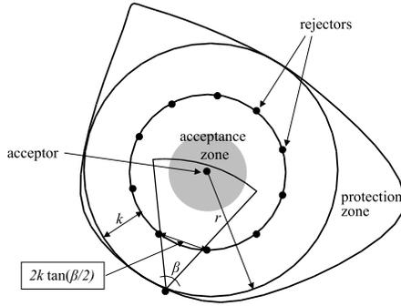
Fig. 4. Placing rejectors to protect against malicious provers with directional antennas. Illustration for the proof of Theorem 4.
